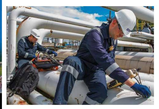
IRISNDT workers perform both guided wave testing (GWT) and ultrasonic thickness testing (UTT) on some piping.
