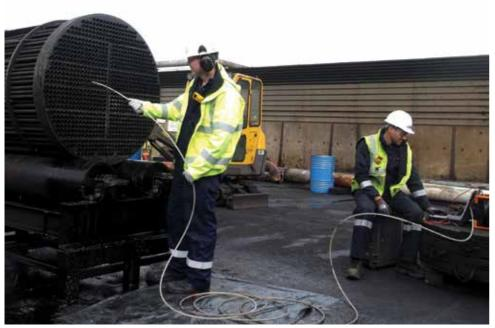
Electromagnetic testing (ET) tube inspection in action.
