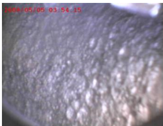
General ID corrosion identified with IRIS. The IRIS indications are shown to the right.
