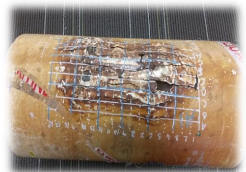
6" line representing the PEC C Scan Above
