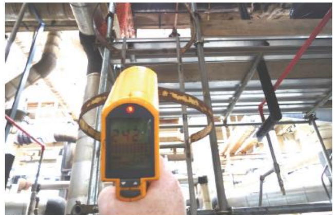
A temperature reading of 242°C (468°F) on the surface of the 8" diesel line.
