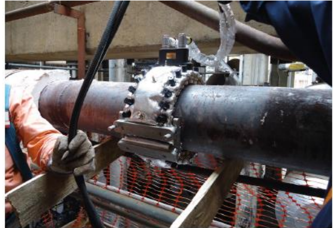
An 8" diesel line operating at 240°C (or 464°F) being tested by a HT inflatable ring.
