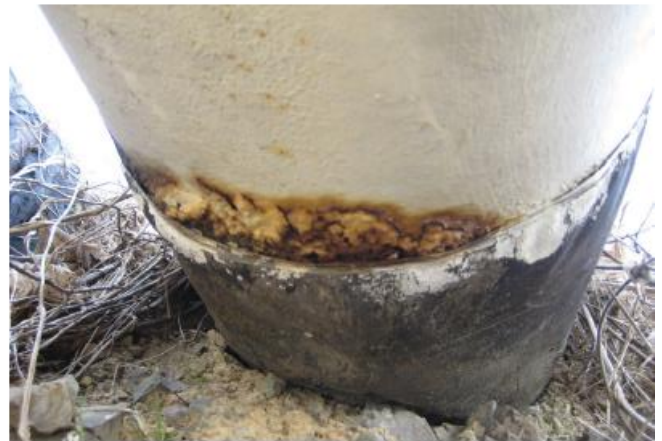
Corrosion patch detected at the entrance location.
