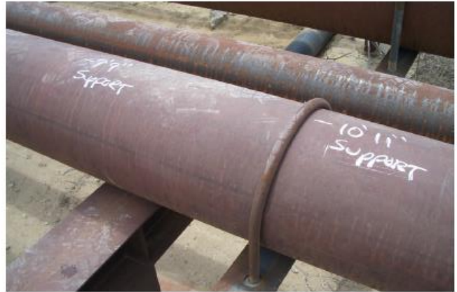
Guided wave testing can screen under sliding and clamped supports.
