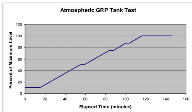
The tank is filled from the start level (50% or less) to the test level. This is usually determined from the tank's maximum operating level for the last year. Load holds (4-minutes each) are incorporated at 50%, 75% and 87.5% with a final hold of 30 minutes at the 100% level. The time taken depends on the size of tank and fill rate, 3-4 hours is typical.
