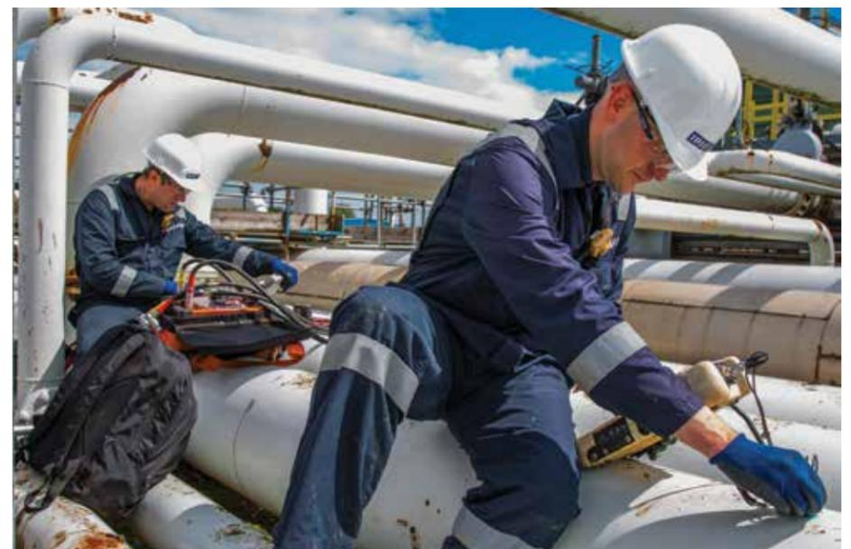
IRISNDT workers perform both guided wave testing (GWT) and ultrasonic thickness testing (UTT) on some piping.
