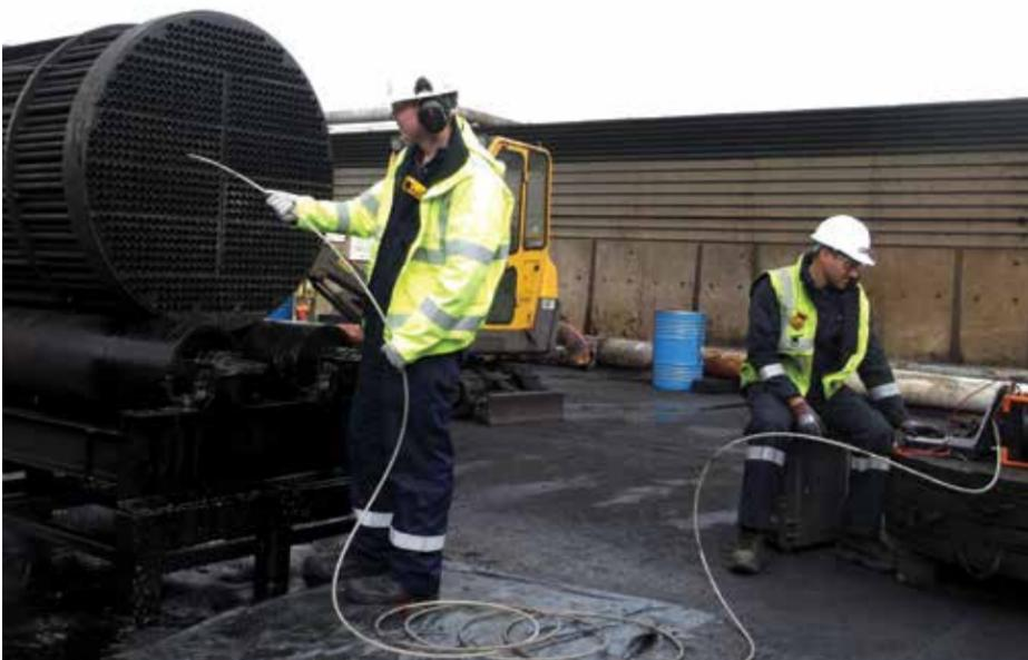
Electromagnetic testing (ET) tube inspection in action.
