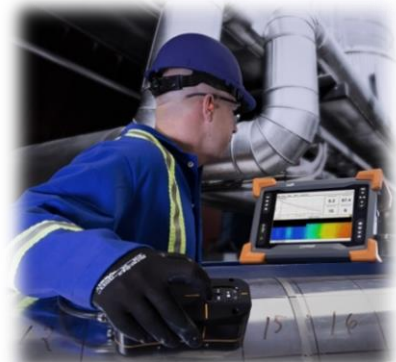
Pulsed Eddy Current system at work
