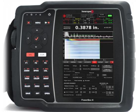
EMAT Scope Displaying Ultrasonic Thickness Readings
