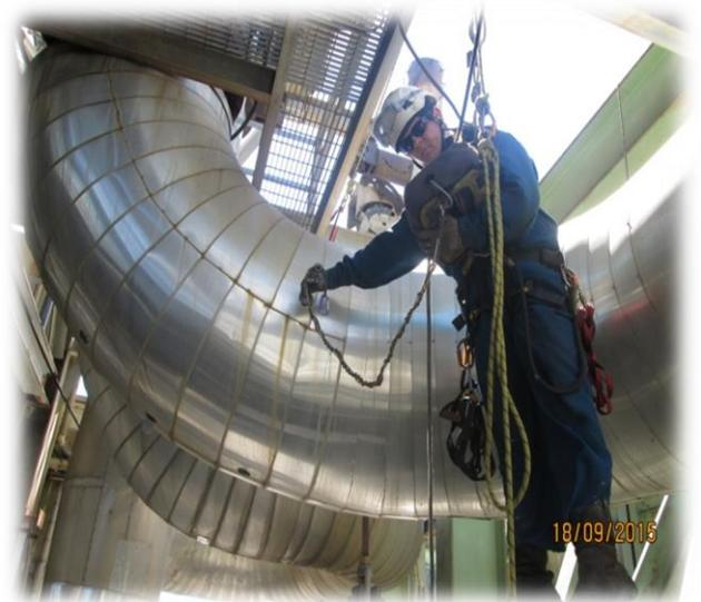
IRISNDT Technician Performing EMAT High Temperature Piping Thickness Measurements While Using Rope Access Technology (Dual Trained Personnel)
