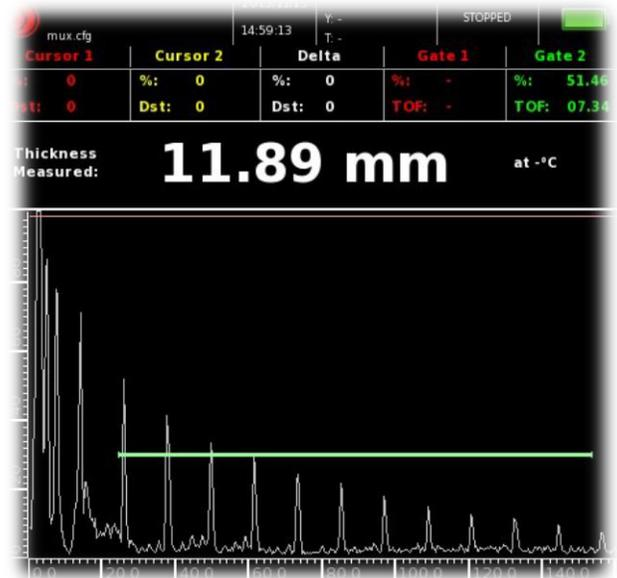
Thickness Measurement – Auto-Correlation Algorithm Represented In Millimeters
