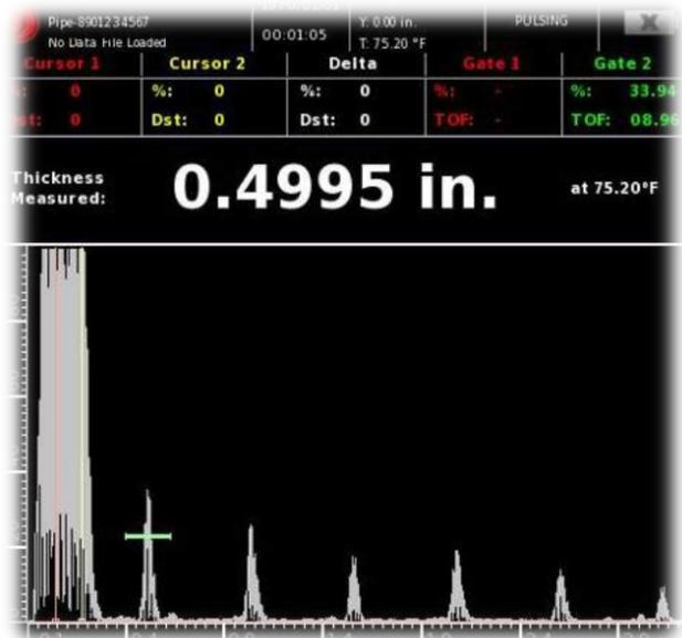
Thickness Measurement – Zero-Crossing Algorithm Represented In Inches
