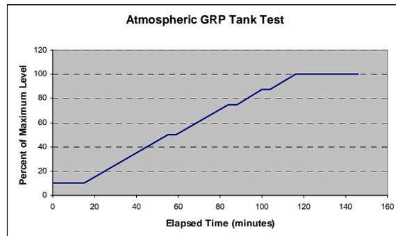
The tank is filled from the start level (50% or less) to the test level. This is usually determined from the tank's maximum operating level for the last year. Load holds (4-minutes each) are incorporated at 50%, 75% and 87.5% with a final hold of 30 minutes at the 100% level. The time taken depends on the size of tank and fill rate, 3-4 hours is typical.
