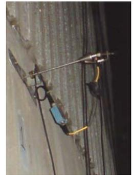
Waveguide Attached to Cladding
