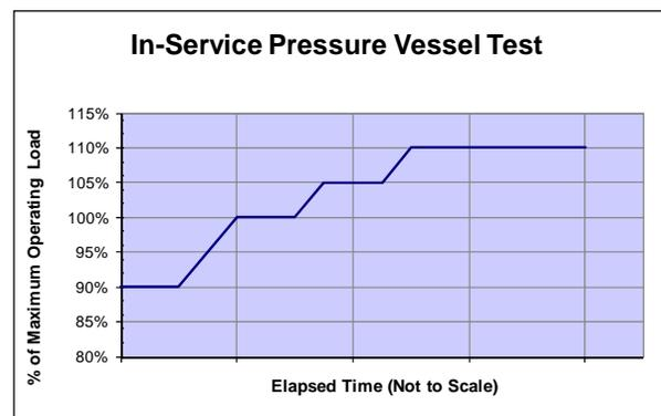
In-service pressure vessels are tested from 90% to 110% of their maximum operating pressure. This may be applied with any suitable medium including nitrogen, process vapor or fluid and water (hydrotest).
